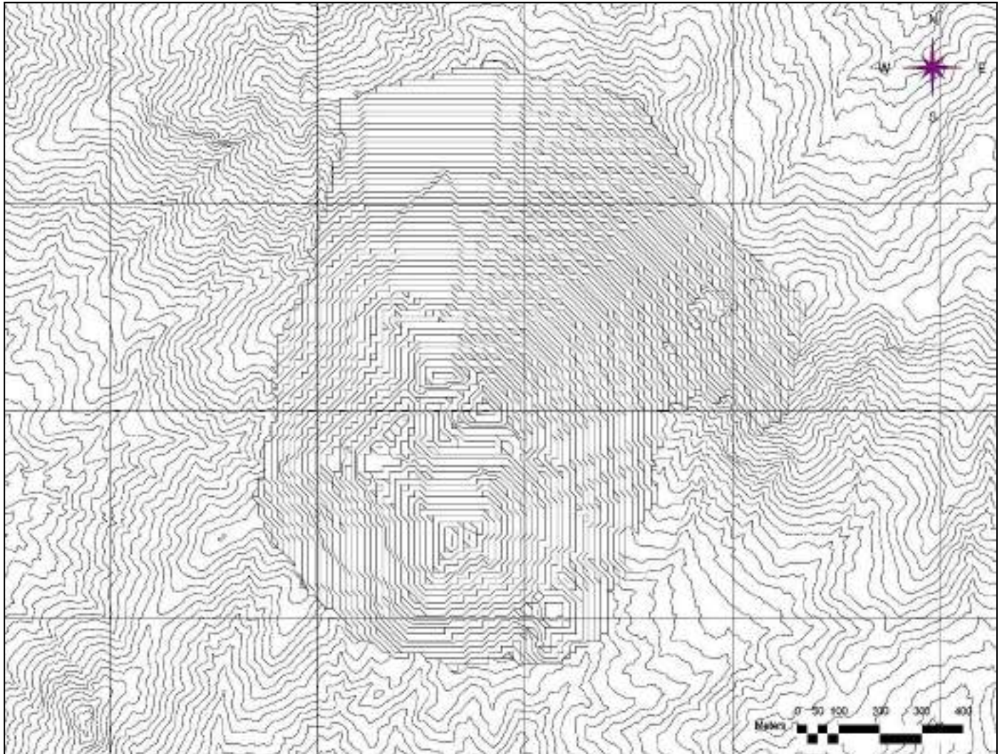
Figure 15-5: Gran Bestia Ultimate LG Optimized Pit (Plan View)
